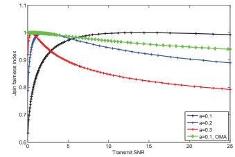
Fig. 4. Jain fairness index versus transmit SNR with different values of a.
