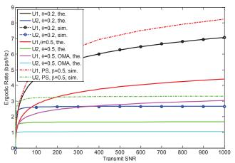
Fig. 2. Ergodic rates versus transmit SNR for UE1 and UE2 with different values of  $\theta$ .
