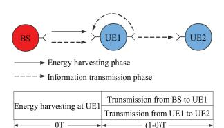
Fig. 1. System model of EH-FD-NOMA and illustration of the TS protocol.
