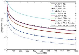
Fig. 3. Outage probability versus transmit SNRs for UE1 and UE2 with different values of  $I_s$ .
